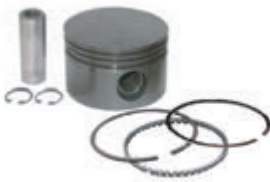
Piston & Segman Set Piston & Ring Set Ø90 mm 2.50 x 2.50 x 4.00 (STD) Ø90 mm 2.50 x 2.50 x 4.00 (0.50) 233-090-103 Ø90 mm 2.50 x 2.50 x 4.00 (1.00) 233-090-105
